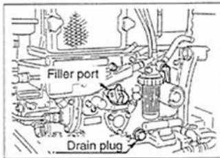
For a new machine, change oil at 20 operating hours for the first time only.
