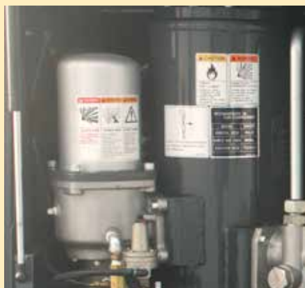
Externally Mounted Separator Filter — Located exterior to the tank and easily serviced by hand for decreased maintenance costs and downtime.
